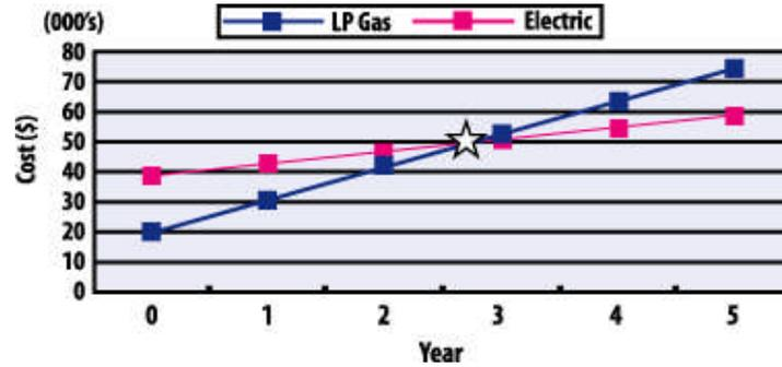
This comparison chart shows the total cost of ownership for electric vs. ICE lift trucks, including the cost of two batteries and one charger at year zero. Over five years, an electric lift truck saves more than 18 percent in total costs.
